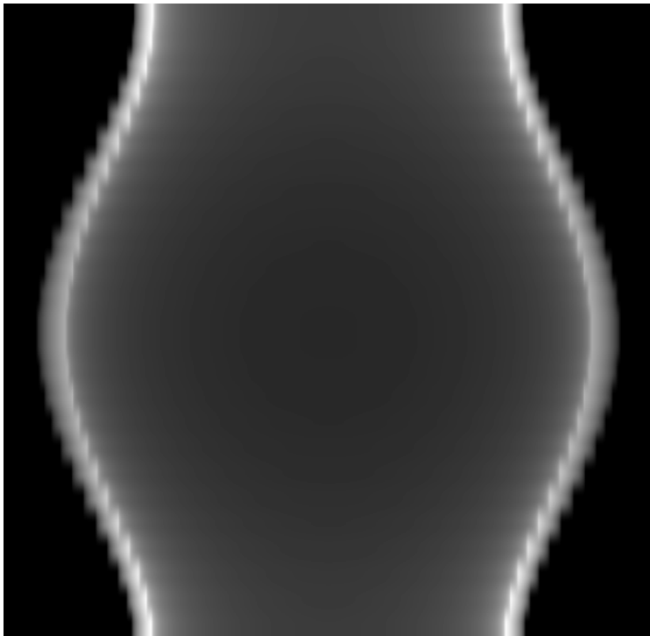
Figure 2: Example of a discrete 2D sinogram
