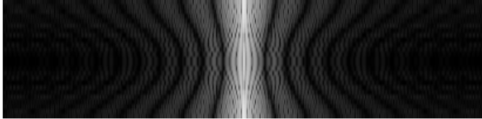
Figure 4: Discrete Fourier Transform of the elliptical phantom's analytical sinogram
